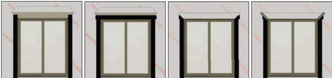
Cut and apply side flashing. Side flashing should run from the bottom of the sill flashing to 4" above the rough opening. Cut and apply head flashing. The head flashing should run slightly past the edge of the side flashing as shown. Flip down the top flap of the house wrap. Tape the cut seams of the house wrap.
