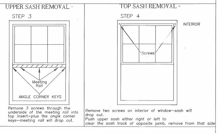
STEP 5 - To reassemble the window simply reverse steps 1 through 5
