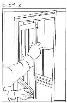
Push the sash to the side into either the right or left sash track of the jamb. allowing the other side of the sash to clear the sash track of the opposite jamb. Remove the sash from that side.
