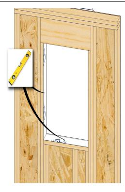
Verify the rough opening is plumb and level. The sill plate beneath the unit must be level for proper unit operation.
