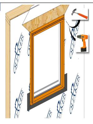
Temporarily fasten with a single fastener at the top of one jamb side as shown.
