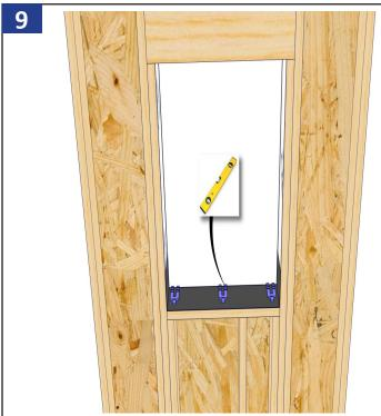
Place shims on the bottom of the opening under each side
