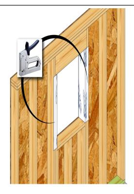
Fold the house wrap to the interior and staple it to the interior framing. Tape the house wrap at the bottom of the opening as shown.
