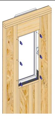
Shim at the sides of the window, and at the check rail locations. Never shim at the head.
