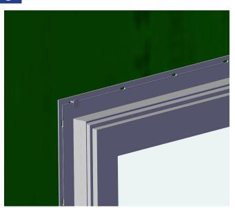
Make sure window is closed and locked before setting the window. Center and set the window into the rough opening, making sure there are equal gaps on both sides of the window.
