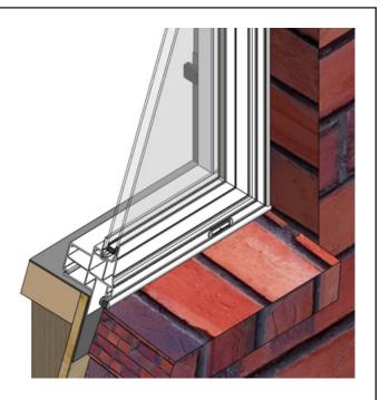
After siding or wall exterior is complete, apply backer rod and sealant between the window frame and exterior finish material on all four sides of unit. Make sure to clean all surfaces before applying sealant.
