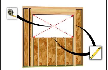
Measure and verify the opening is sized correctly. The rough opening should be a minimum 1/2" (but not to exceed 1") wider and taller than the unit. Allow additional space for flashing thickness, installation clips, joining components, and their fasteners.
