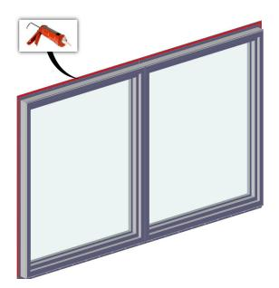
Apply a 3/8" diameter bead of 100% neutral cure silicone sealant (ASTM C920 compliant) along the backside of the nailing flange.
