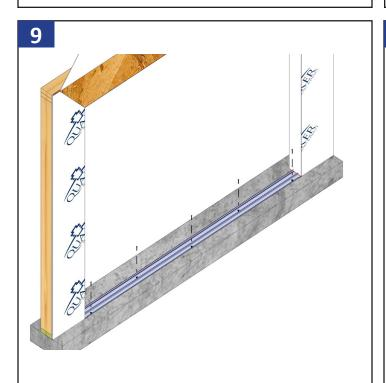
Fasten sub-sill anchor plate as shown above.
