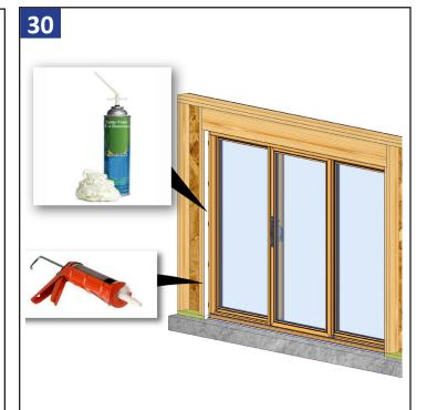
Fill interior 1/3 of cavity using low expanding foam or backer rod and apply sealant continuously around entire perimeter of opening.
