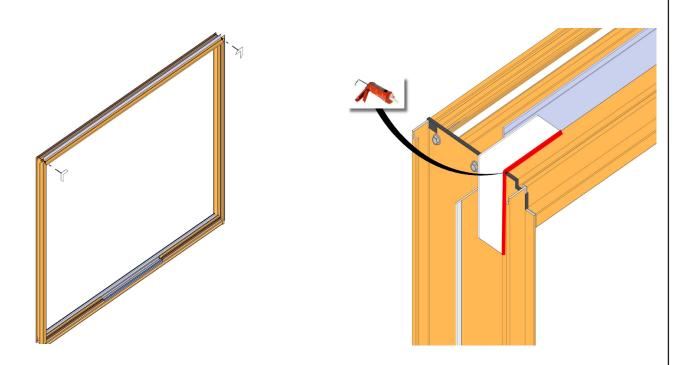
Clean the nail fin corners with 99% isopropyl alcohol prior to installing the corner gaskets to the exterior side of nail fin corner gaps. Apply sealant along the edge where the gasket meets the door frame as shown.
