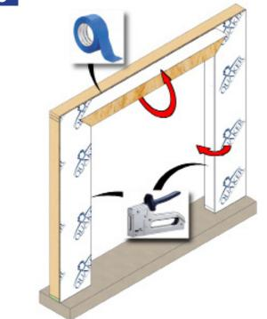
Fold the house wrap around the jambs to the interior and staple it to the interior framing. Fold the house wrap flap up and temporarily tape it in place.
