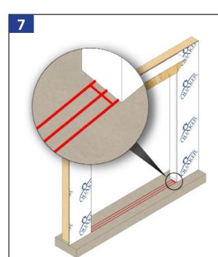
The sub-sill anchor plate will set 4 1/16" in from the exterior face of wall framing. Apply three 3/8" continuous beads of sealant across the entire width of the rough opening sill where the sub-sill anchor plate will set. Apply two 3/8" continuous beads of sealant the depth of the anchor plate, 1/2" from each side of opening as shown above.
