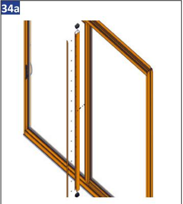
If reinforcement tube is to be applied, center the reinforcing tube on the active panel's meeting rail, and install using supplied (MH8-18x1/2 TK2) screws.
