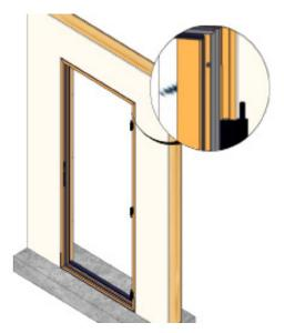
Install and fasten the door unit in place using fasteners by others per anchorage calculations. *Quaker Window Products does not supply or claim liability for anchorage/fastener calculations. It is the installer/client's responsibility for structural adequacy of the anchorage and fasteners.* Typically, 3" from the corners and 16" on center, and at every hinge and lock location.
