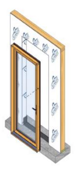
Center and set the door frame into the rough opening. Make sure to keep the door flush with the interior wall finish. Level at the sill and plumb the frame. Shim under the frame to bring to level in necessary.
