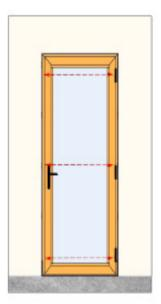
Verify the door is square, level, and plumb. Check the spacing around the door at the top, middle, and bottom to make sure the door is not over shimmed. See hinge and lock adjustment guides if adjustments are needed.
