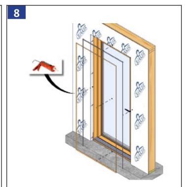
Apply backer rod as needed and a continuous bead of sealant around the entire perimeter of the door unit.
