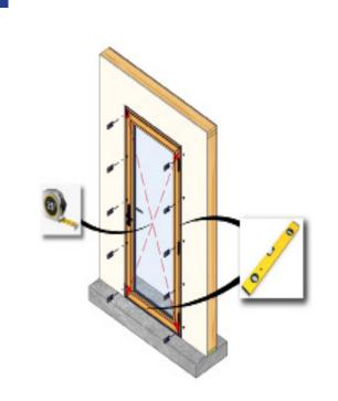
From the interior, square the frame in the opening by installing shims between the jambs and framing.
