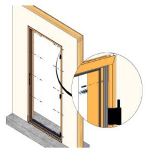
Drill a countersink hole through the jambs in the exterior track per anchorage calculations. Quaker Window Products does not supply or claim liability for anchorage/fastener calculations. It is the installer/client's responsibility for structural adequacy of the anchorage and fasteners.
