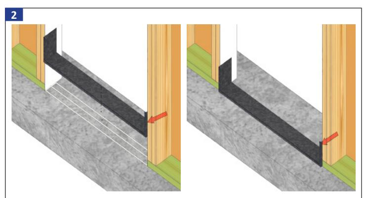
Install a sill pan flashing (by others). If installing the door flush with the interior to allow for a 180 degree door swing make sure to set the sill pan flush with interior wall finish.
