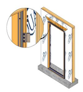
Install and fasten the door unit in place using fasteners by others per anchorage calculations. Typically, a #12 screw 6" from the top and bottom and 16" on center thereafter. Always follow the anchorage calculations and fastener/ anchor manufacture's guidelines for proper edge distance, load capacity and installation techniques.
