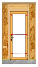
Verify the door is square, level, and plumb. Check the spacing around the door at the top, middle, and bottom to make sure the door is not over shimmed.
