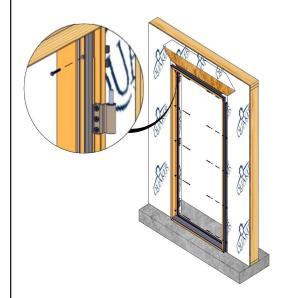
Drill a countersink hole through the jambs in the exterior track per anchorage calculations. Quaker Window Products does not supply or claim liability for anchorage/fastener calculations. It is the installer/client's responsibility for structural adequacy of the anchorage and fasteners.
