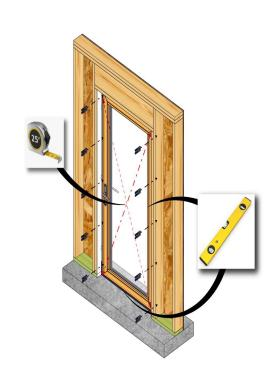
From the interior, square the frame in the opening by installing shims between the jambs and framing.
