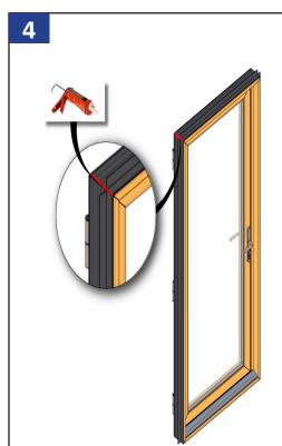
Snap the fin into place with short side of the flange facing the exterior. Seal the corners of the position fin.
