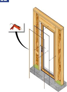
Apply insulation and a continuous bead of sealant around the entire interior perimeter of the door unit.
