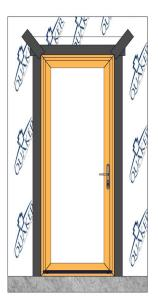
Flip down upper flap of WRB so it lays flat across head flashing, then trim 1" - 2" above the door opening. Tape along all cuts in WRB and across head of the door with flashing tape.
