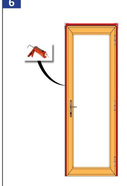
Install a continuous bead of sealant around the interior side of the position fin.
