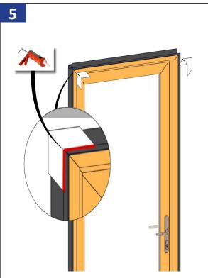
Install the two top foam corner key gaskets over the exterior side of the position fin corner gaps. Seal the exterior corners where the foam gasket meets the position fin.
