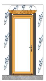
Cut two pieces of flashing tape for jamb flashing extending 1" above head position fin. Remove release paper and press tightly along sides of door frame.
