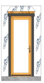
Cut a piece of flashing tape for the head flashing, which extends beyond outer edges of jamb flashings. Remove release paper and install completely covering position fin and adhering to exposed sheeting or framing members.
