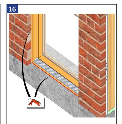
Apply a continuous bead of sealant across the full length of the sill and around exterior perimeter of door unit.
