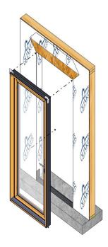
Center and set the door frame into the rough openings pushing the position fin tight against exterior framing.
