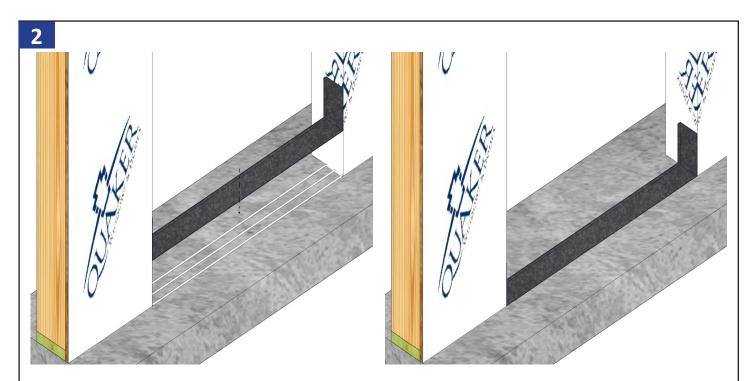
Install a sill pan flashing with minimum 1/2" interior leg (**by others**). If installing the door with the position fin set the sill pan  $3 \ 3/16$ " in from the exterior.
