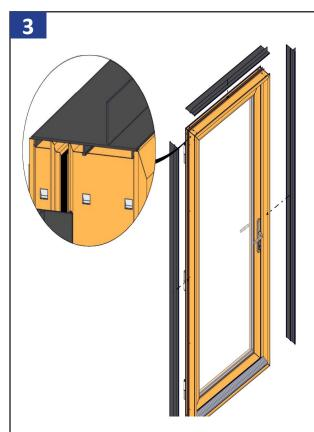
Install the position fin onto the frame if not installed at the factory on the head and both side jambs.
