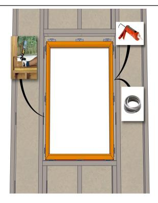
Apply sealant continuously around entire perimeter of opening, filling interior 1/3 of cavity using low expanding foam or backer rod and sealant.
