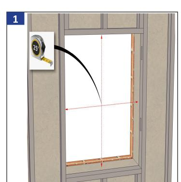
Measure and verify the opening is sized correctly. The rough opening should be a minimum 1/2" (but not to exceed 1") wider and taller than the unit. Allow additional space for flashing thickness, installation clips, joining components, and their fasteners.
