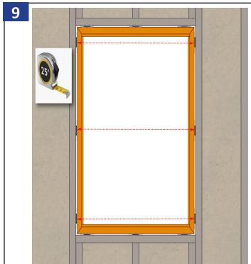
Check that the window is not bowed. Adjust shims as needed until measurements are within 1/8".
