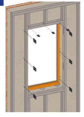
Shim at the sides of the window, and the check rail locations. Make sure to shim the window and the backside of the anchor straps.
