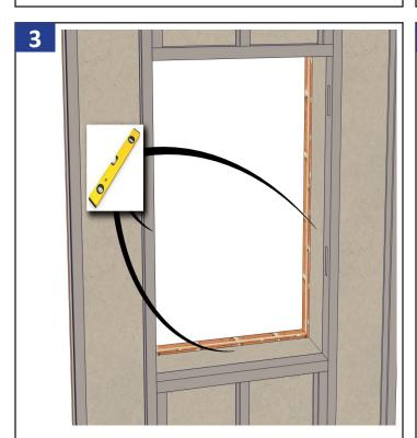
Verify the rough opening is plumb and level. The sill plate beneath the unit must be level for proper unit operation.
