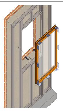
Set the window in place on top of the shims at the sill, and center in opening.
