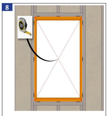
Check that the window is square. Adjust shims as needed until diagonal measurements are within 1/8".
