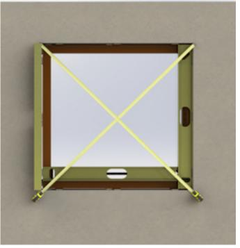
Set the window in place on top of the shims at the sill, and center in opening. Place a level on the window sill to verify that the sill is level. Adjust the shims as needed to ensure a level condition. Check the head, sill and jambs with a level again to make sure the window is setting plumb, level, and square within the opening. Measure across the diagonals to determine if the window is square.
