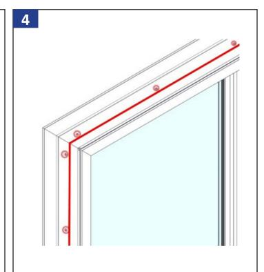
Apply sealant along the edge of the flush fin casing against the interior unit side and on each screw head. Install the unit per the thru jamb window installation guide.
