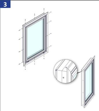
Screw the flush fin casing to unit using provided screws. Place screw 2" from each end and 8" on center. Keep screws to the interior side for flush fin casing.
