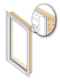
Apply a screw in each of the top corners of the BMC to hold the mitered corners together.
