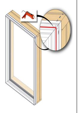
Apply a small amount of sealant inside the mull kerf at the head and down both side jambs.
