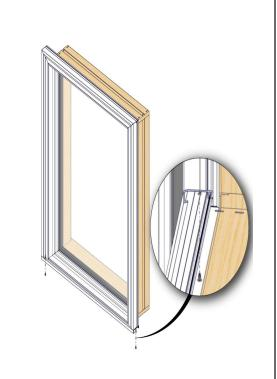
Install two screws through the sill nose into the BMC screw boss as shown above.
