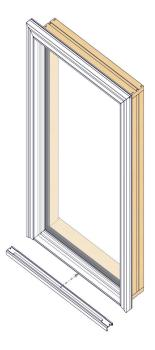
Apply a small amount of sealant into the inside of the sill mull kerf. Align sill nose and snap into the mull kerf.
