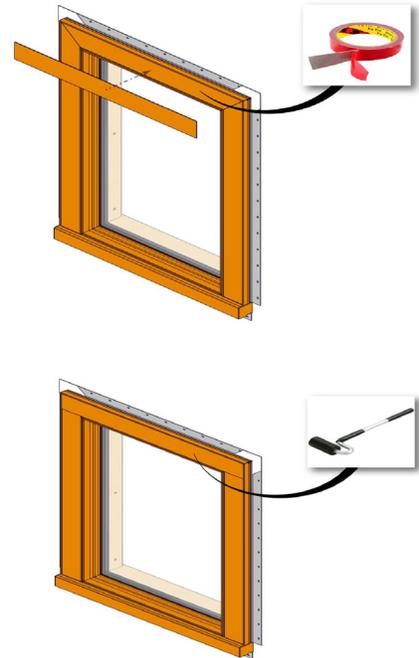
Apply two strips of double sided tape the full length of the top and apply the break metal cover for the squared BMC look. Use a J-roller and apply pressure to ensure a good bond.
