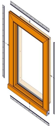
If using the nail fin snap it into the kerf on the BMC and sill nose.
