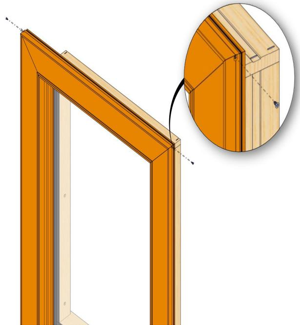
Apply a screw in each of the top corners of the BMC to hold the mitered corners together.
