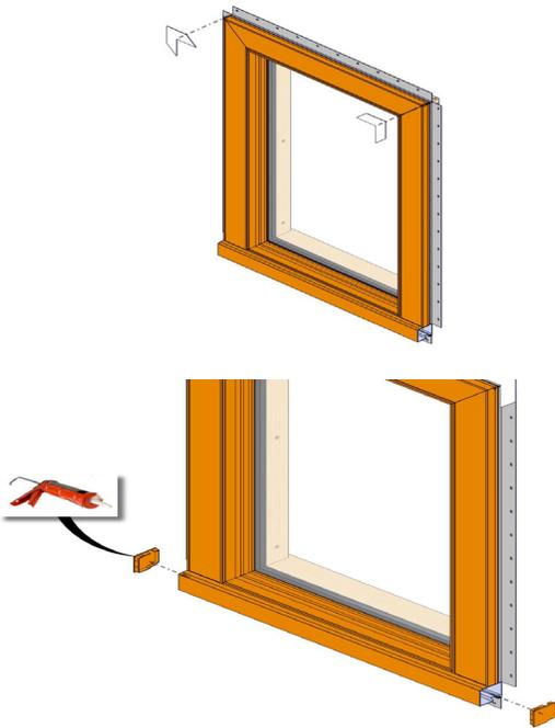
Install the top corner nail fin gaskets as shown above.
