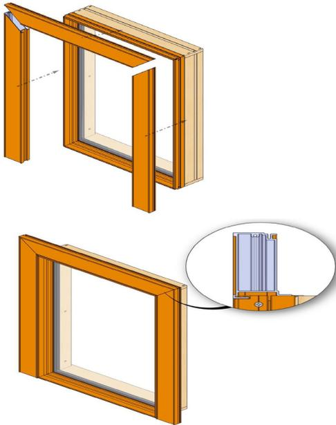
Align the head BMC and snap it into place. Align the side jambs and snap into place.
