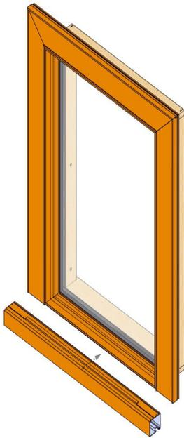
Apply a small amount of sealant into the inside of the sill mull kerf. Align sill nose and snap into the mull kerf.
