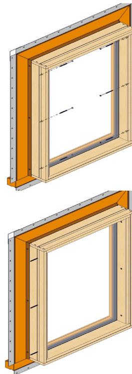
Wide BMC requires the installer to anchor the windows through the jambs or to use anchor straps.
