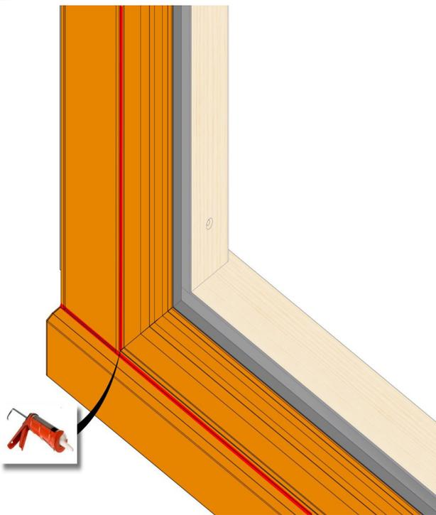
Apply a cap bead of sealant along all edges and corner where the BMC meets the window.
