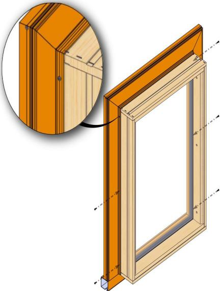
Install self tapping screws around the perimeter of BMC attaching it to the window frame as shown above.
