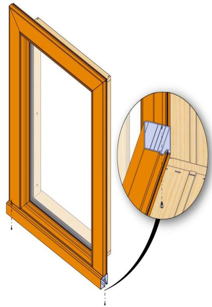
Install two screws through the sill nose into the BMC screw boss as shown above.
