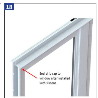
After unit is installed in wall, install drip cap over the nail fin the full length of mulled units at the head. Notch the drip cap ends if necessary for standard J-channel installation practices.
