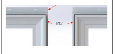
Using a utility knife score and remove all but 5/32" of the nailing fin from each unit where the mull will connect them. Make sure to cut the head and sill nail fins back flush with ripped nail fin as shown above.
