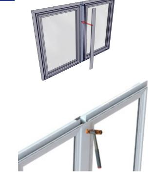
Install the mull key flush with one side of unit and hammer into place with rubber hammer.
