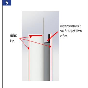
Apply a continuous bead of sealant down both edges of the mulled side of the window and across the top and bottom.
