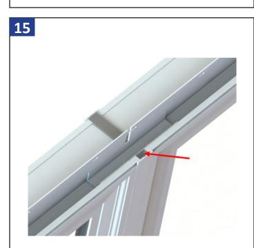
Apply sealant to the bottom edge of the jamb filler before installing it in the j-channel pocket at both ends of mullion, and add sealant to gap between filler and mull key.
