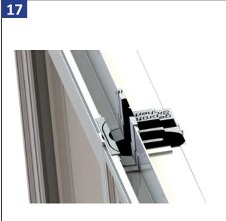
Apply self-adhesive flashing tape over the top side of mull gap and over nail fin.
