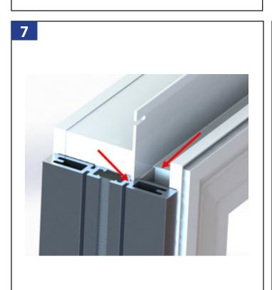
Apply the mullion to the side of the window aligning the groove in the mullion with the cut down nail fin. Make sure the mullion doesn't stick pass the j-channel pocket. Press firmly to engage the double-sided tape.
