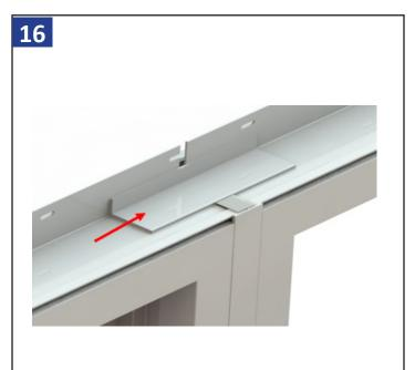
Apply 5"-7" piece of nail flange filler to interior back side of nail fin in a bed of sealant.
