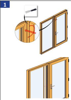
Set Hinged door in the opening per standard installation guides. Install fasteners through jamb of door to hold door in place. Remove vertical then top glass stops of side-lite using a putty knife.
