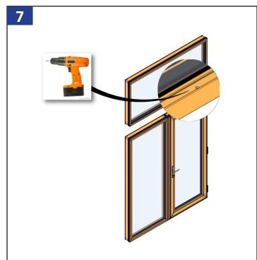
Remove vertical then bottom glass stops of transom. Predrill holes in jamb for #8 screws to attach mull #57588 3" from top and bottom and 16" on center thereafter.
