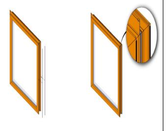
Clean the frame legs before applying the tape gaskets to the interior and exterior legs of one of the mulled units as shown above. 4
