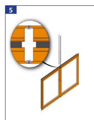
Cut the C-mull keys to the length of the unit. Install the mull key from the top or bottom sliding the mull key the full length of windows locking them together as shown above. You may need a block and hammer to drive the mull keys in.
