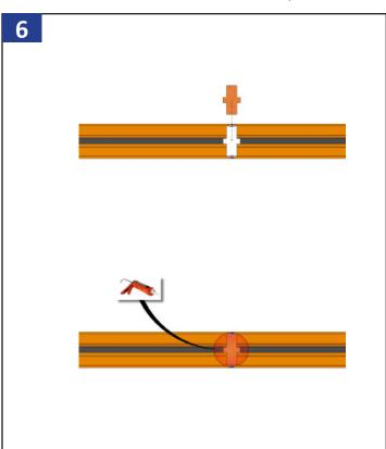
Cut a foam plug to fill the gap between the units at the head and sill. Once foam plugs are in place cover with sealant and tool flat as shown above.
