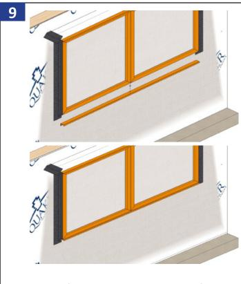
Apply a bead of sealant along the bottom exterior frame leg and set the sill flashing the full length of units as shown above.
