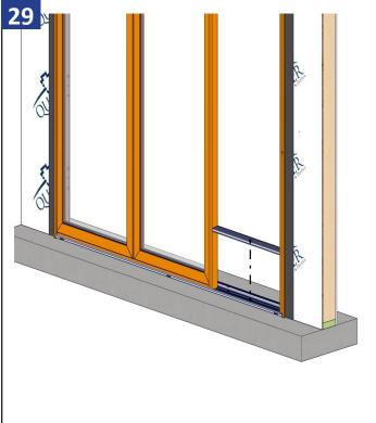
Install threshold on the exterior side of frame covering the bottom angle brackets.
