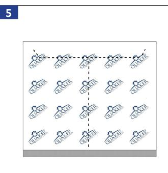
Apply the house wrap according to the manufacturer's instructions and cut T-pattern opening as shown above. Cut top flap angles at 45 degrees and 1" longer than the width of flashing tape being used.
