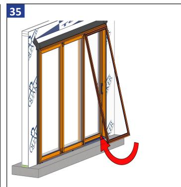
Angle the screen panel with the top inserted into the head track, and then lift and set the bottom rollers on the roller track. Adjust rollers as needed to insure the panel is level, square, and slides smoothly.
