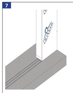
Apply three 3/8'' continuous beads of silicone across the entire width of the rough opening sill, and a 3/8'' continuous bead of silicone  $\frac{1}{2}''$  from each side of the rough opening as shown above.
