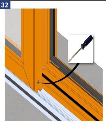
Adjust the rollers as needed to insure the panel is level, square, ans slides smoothly.
