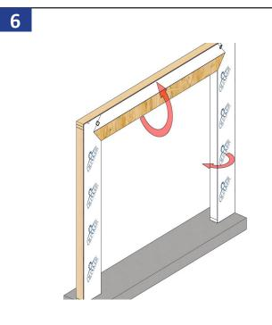
Fold the house wrap to the interior and staple it to the interior framing. Fold the house wrap flap up and temporarily tape it in place.
