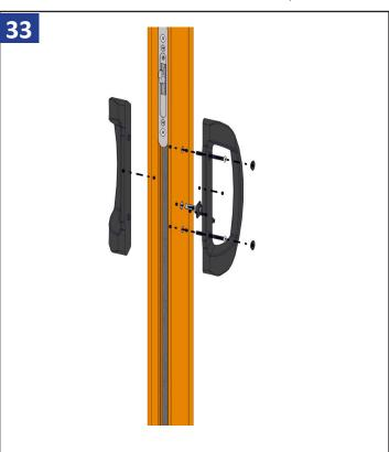
Install handle set using provided instruction found in the hardware box using the 1 7/8" door thickness section.
