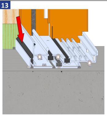
Install the wedge gasket in the sub-sill anchor plate against the interior leg of the door as shown above.
