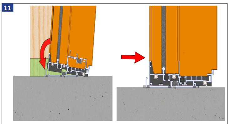
Center and set the door frame into the rough opening, making sure there are equal gaps on both sides of the door. Angle the door frame with the top tilted out, and set the exterior sill frame inside the exterior leg of the sub-sill anchor plate as shown above. Push the frame in against the framing locking the sill into the sub-sill anchor plate.
