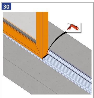
Seal around the two ends of the threshold against the frame as shown above.
