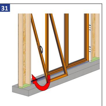
Angle the active panel with the top inseted into the head track, and then lift and set the bottom rollers on the roller track.
