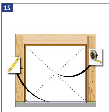
Check that the door is square. Adjust shims as needed until diagonal measurements are within 1/8". Level at the sill and plumb the frame.
