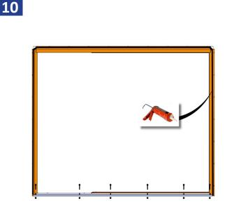
Apply a continuous 3/8" diameter bead of sealant along the backside of the nailing flange. Bead must run around both sides and across the head, in line with and completely covering the nail flange holes.
