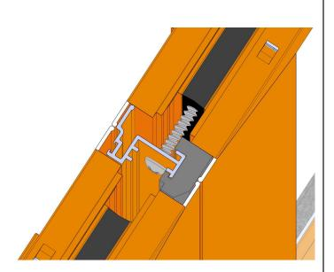
Slide the astragal side of the panel tight against the first fixed panel keeping the panel flush with the fixed panel extrusion in the sill.
