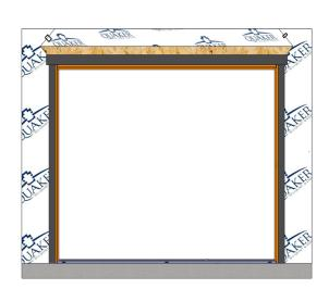
Apply a 3/8" sealant bead to the top exterior edge of door frame before installing the drip cap.
