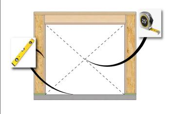
Measure and verify the opening is sized correctly. The rough opening should be a minimum 1/2'' (but not to exceed 1'') wider and taller than the unit. Allow additional space for flashing thickness, installation clips, joining components, and their fasteners.
