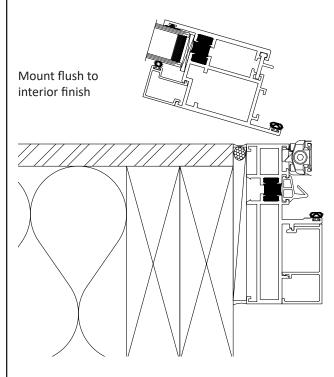
For inswing units where full panel operation is desired, install the unit flush with interior finish surface of wall.
