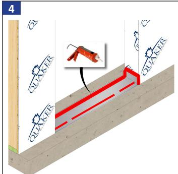
Apply a continuous bead of sealant to the exterior face of the upturned leg of the sill pan. Also seal where the sill pan flashing meets the rough opening, and tool sealant over any fasteners used to install the pan.
