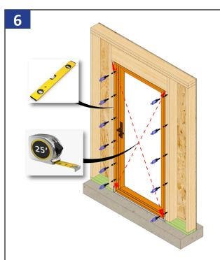
Square, level, and plumb unit in the rough opening by applying shims as needed. Shim behind all hinges and lock points, do not over shim, do not shim at the head.
