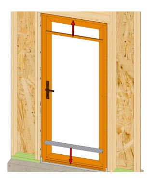
Install the jamb covers, then the head cover and threshold.
