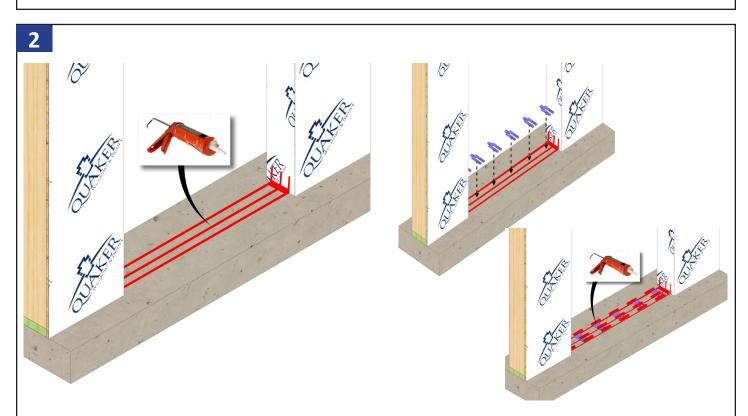
Apply three continuous 3/8" beads of sealant on the sill where the pan flashing will set. Also generously apply sealant along the bottom corners of the rough opening. Set shims in the bed of sealant and apply additional sealant over the top of the shims.
