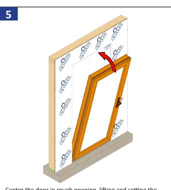
Center the door in rough opening, lifting and setting the bottom of the door in first, then tilting into place.
