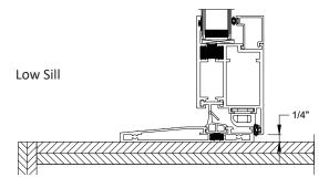
The panel must clear interior finishing material for proper operation. If the interior finishing material is greater than 1/4" for low sill units, or 15/16" for all other inswing units, raise door unit by placing waterproof shims or spacer under sill to gain sufficient clearance.
