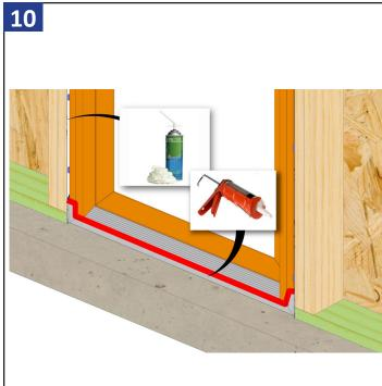
Apply a bead of sealant to fill the gap between the sill pan flashing system and the interior of the door unit. Make sure to seal all the way up both ends of the corner mold against the door.
