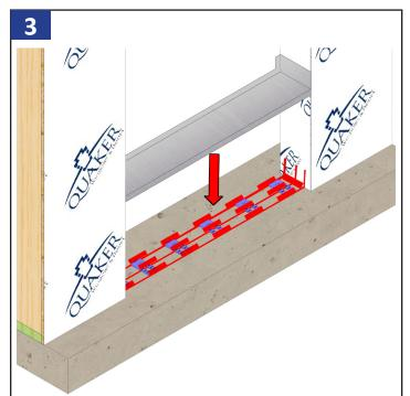
Apply sill pan flashing. The flashing must extend to the exterior face of the wall.
