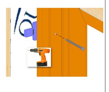
Drill a pilot hole through the jamb's walls per anchorage calculations. *Quaker Window Products does not supply or claim liability for anchorage/fastener calculations. It is the installer/client's responsibility for structural adequacy of the anchorage and fasteners*. Typically, a #12 screw 6" from the top and bottom and 16" on center thereafter. Install and fasten the door unit in place using fasteners by others per anchorage calculations.
