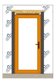
Cut two pieces of flashing tape for jamb flashing extending 1" above the head positioning fin. Apply flashing tape and smooth using J-roller.
