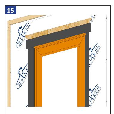
Apply flashing tape over the drip cap leg, overlapping the side flashing as shown. Smooth using a J-roller.
