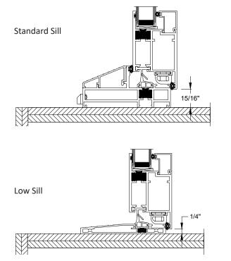
The panel must clear interior finishing material for proper operation. If the interior finishing material is greater than 1/4" for low sill units, or 15/16" for all other inswing units, raise door unit by placing waterproof shims or spacer under sill to gain sufficient clearance.
