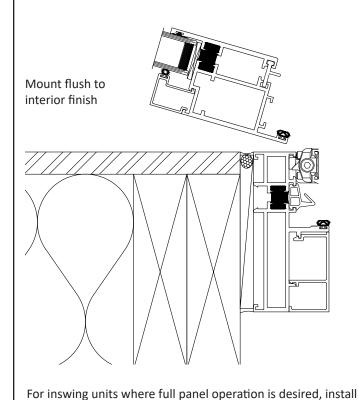
the unit flush with interior finish surface of wall.
