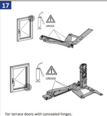
Clean top and bottom hinges thoroughly and apply white lithium grease to the hinges. This should be done twice a year. Recommended spring and fall.
