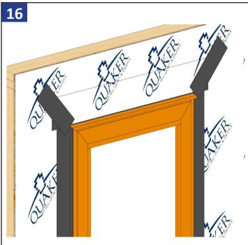
Flip down upper flap of the weather resistant barrier so it lays flat across head flashing and tape the angle cuts as shown above.
