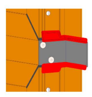
Use silicone to seal the entire area between the stack mull and top/bottom units. Do this for both sides of the mull.
