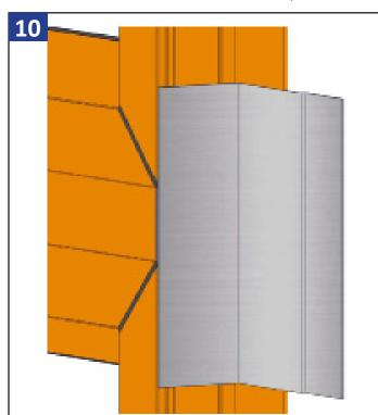
Apply self-adhesive flashing tape over the mull area and nail fins.
