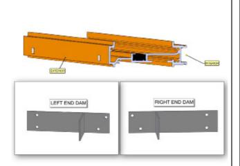
Note the orientation of the stack mull interior and exterior sides. Exterior side will have weep slots. Note orientation for the end dams (left and right as seen from the exterior side of the window).
