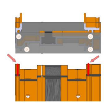
Apply two continuous beads of silicone on top of the first unit, the full length of the unit as shown. Set the stack mull on top of the first unit.
