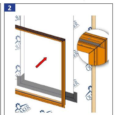
Install the bottom unit in place following the QWP standard nail fin installation guide. Check the unit has the nail fin removed on the top side where the stack mull will go.
