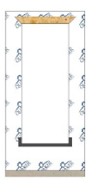
Prepare the rough opening per the QWP installation guideline for nail fin applications.
