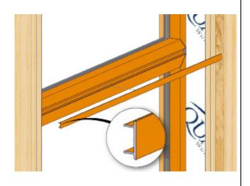
Snap into place the interior aluminum snap cover to complete mull install.
