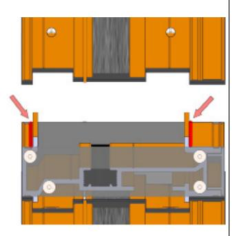
With the stack mull in place, apply two continuous beads of silicone on top of the mull along its full length as shown. Set the second unit on top of the stack mull.
