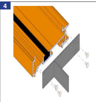
Install the end dam on the end of the stack mull using the 4 included pop rivets (right side shown). Repeat for the other end of the stack mull.
