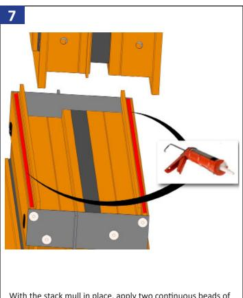
With the stack mull in place, apply two continuous beads of silicone on top of the mull along its full length as shown. Set the second unit on top of the stack mull.
