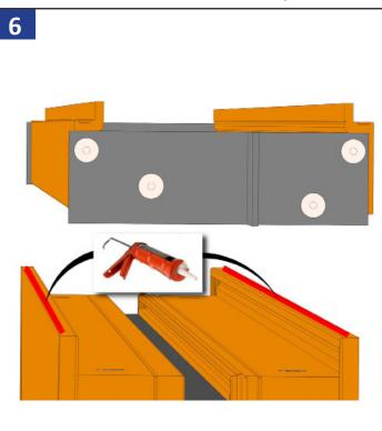
Apply two continuous beads of silicone on top of the first
