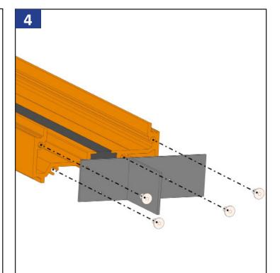
Install the end dam on the end of the stack mull using the 4 included pop rivets (right side shown). Repeat for the other end of the stack mull.
