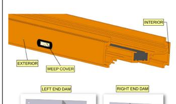
Note the orientation of the stack mull interior and exterior sides. Exterior side will have weep slots. Note orientation for the end dams (left and right as seen from the exterior side of the window).
