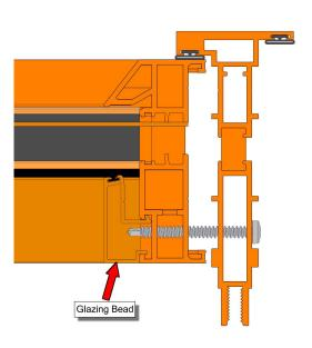
Drill pilot holes through the transition mull into the window/sidelite unit. Fasten through the mull into the window/sidelite, typically with #12 x 2" screws by others, spaced 6" from the top & bottom and 16" centers thereafter.
