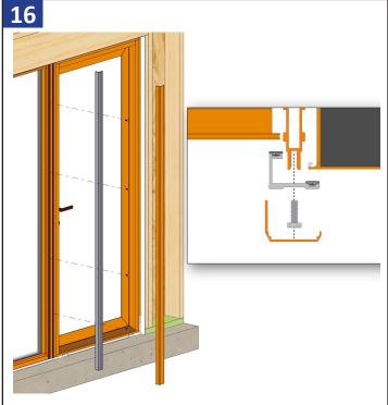
Insert the base plate with the weather-strip flat against the window and door units and install with supplied bolts (MH14 20x3/4) approximately 18" on center. Snap the finish trim cap over the base plate to finish the T-mull.
