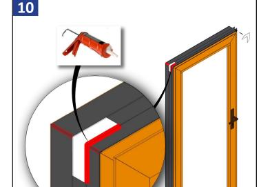
Install the top foam corner key gasket over the exterior side of the positioning fin corner gap on the door. Seal the exterior corner where the gasket meets the position fin as shown above.
