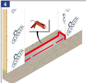
Apply a continuous bead of sealant to the exterior face of the upturned leg of the sill pan. Also seal where the sill pan flashing meets the rough opening, and tool sealant over any fasteners used to install the pan. Apply a discontinuous bead of sealant across the front of the sill pan flashing where the front of the unit will sit.
