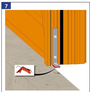
**For all Installations:** Verify transition mull is vertical and centered properly between the units being installed. Install L-angle at the sill in a bed of sealant with fasteners into sill, per shop drawings or anchorage calculations. Secure the L-angle to the transition mull at the sill with two self-tapping screws supplied by others, typically #12 x 1" screws.
