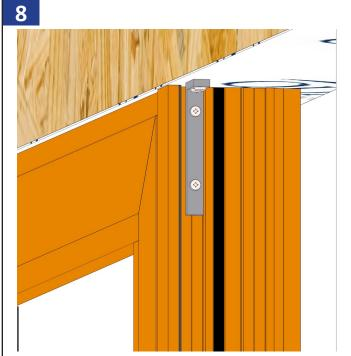
For Installations without Positioning Fin on Door and No Nail Fin on Window: An anchor clip is not used at the header. Verify the transition mull is spaced properly and vertical. Install the L-angle with fasteners into header, per shop drawings or anchorage calculations. Secure L-angle to the mull with self-tapping screws, typically #12 x 1" screws.
