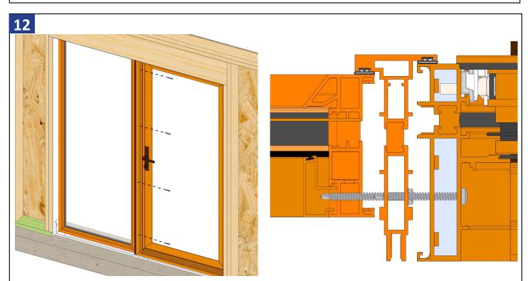
Drill pilot holes through the door jamb into the transition mull. Fasten through the door jamb into the mull, typically with  $#12 \times 2$ " screws by others, spaced 6" from the top & bottom and 16" centers thereafter. Jamb cover, head cover and sill threshold can now be installed on the door.
