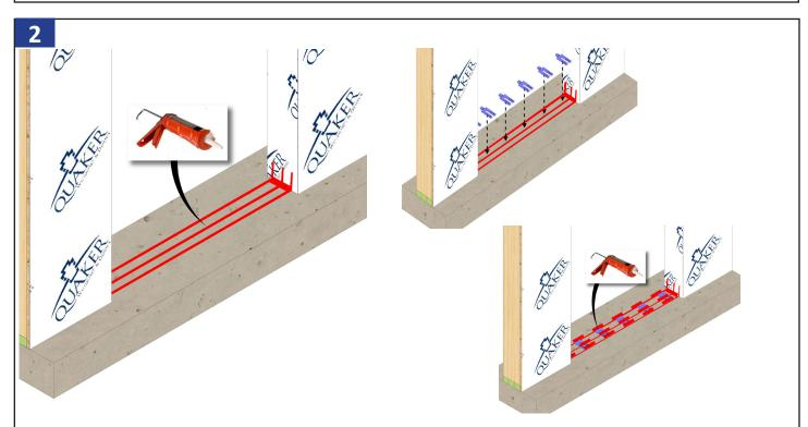
Apply three continuous 3/8" beads of sealant on the sill where the pan flashing will set. Also generously apply sealant along the bottom corners of the rough opening. Set shims in the bed of sealant and apply additional sealant over the top of the shims.
