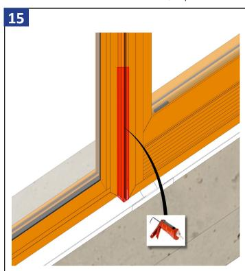
Apply sealant, on the interior side, up the bottom 6" of the center of the transition mull filling the entire area as shown.
