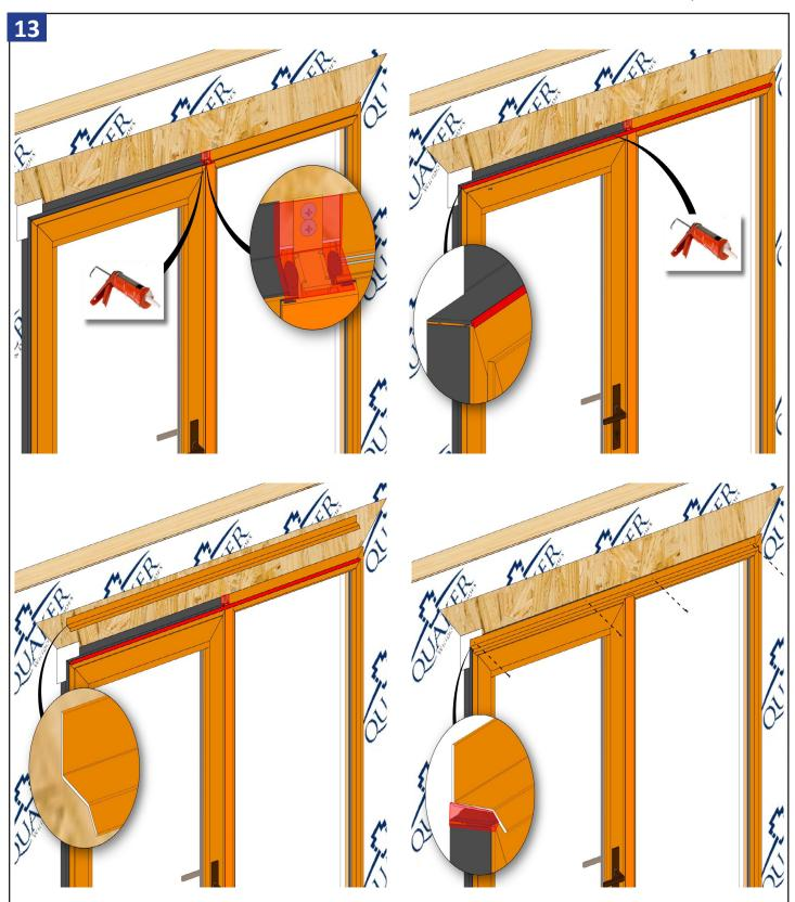
After units and mulls have been installed, leveled, and squared, insert backer rod into gaps between frames at the top of the mull. Apply sealant over the top of the transition mull area to cover gaps between the mull and frame. Apply a continuous bead of sealant across the entire top outer frame edge then set drip cap and fasten in place. Use backer rod and sealant to cover both ends between the drip cap and frames.
