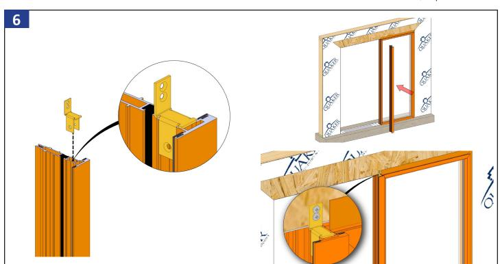
Install the anchor clip in the top of the T-mull as shown above. Install the transition mull so the anchor clip is to the exterior. Verify the mull is vertical and located in the opening with proper spacing between the door and window units per shop drawings (e.g. 1" spacing between door and window with a 1" mull). Fasten the mull anchor to the header on the exterior wall, typically with #12 x 1" screws supplied by others, per anchorage calculations or shop drawings.
