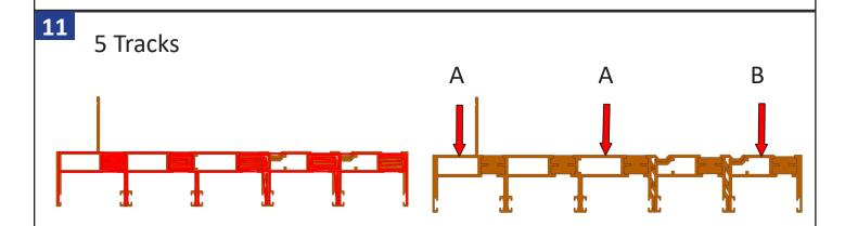
Place a gasket (Part #: QWP-MMSD-V5FG5(B/W)) on each face profile of the frame header. Place 2 of the corner keys (Part #: FE\_25-7x10-35-DT) in both ends of the frame header by arrow (A) and place corner key (Part #: M25762-PCS) by arrow (B). Then join to both frame jambs to head. Trim weather strip flush to both ends.
