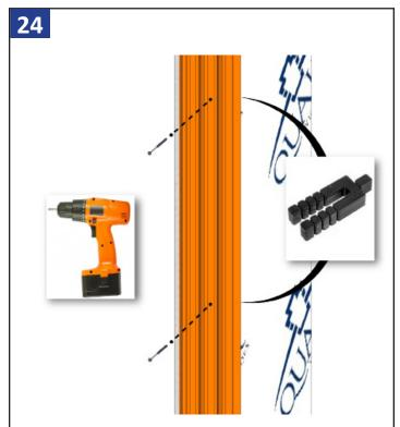
Temporarily set screw just deep enough to hold the frame in place. The screws through the center track of the header & jambs, typically 6" from ends and 24" on center for fasteners.
