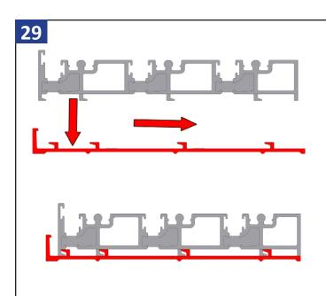
Push the sill down and then toward the exterior to lock in the sill to the sill pan.
