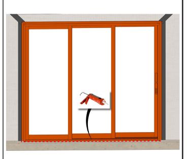
Apply a continuous bead of sealant at the exterior base of the sill. Be sure to not block the weeps on the bottom of the sill.
