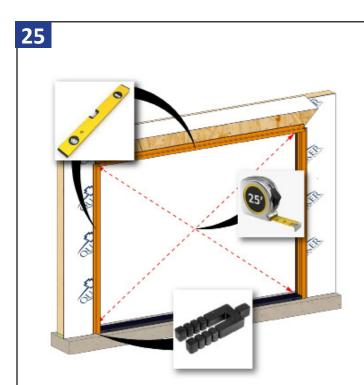
Square, level, and plumb the frame. Adjust shims as needed until diagonal measurements are within 1/8". Shim behind the header and jambs as necessary.
