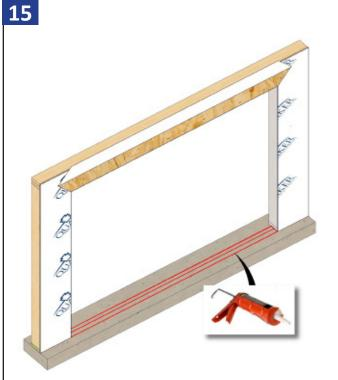
Apply three 3/8" continuous beads of sealant across the entire width of the rough opening sill where the sill pan will set. Apply two 3/8" continuous beads of sealant the width of the pan, 1/2" from each side of opening as shown above.
