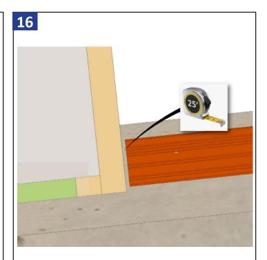
Allow a 1/4" gap between the rough opening and the sill nan(s)
