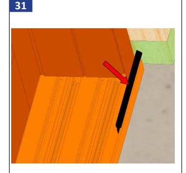
Cut a small piece of wedge gasket and place it in the center, as well as, one piece at each end.
