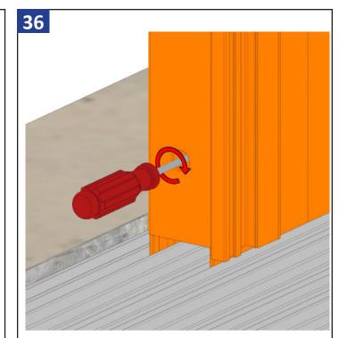
Use a #2 phillips screwdriver to engage the roller adjustment on both sides of a panel. Turn clockwise to raise the panel and provide smooth rolling. If possible, lift the panels slightly when adjusting to take pressure off the rollers. Roll panel back and forth 2-3 times to verify roller height is set. Repeat this step for each panel installed.
