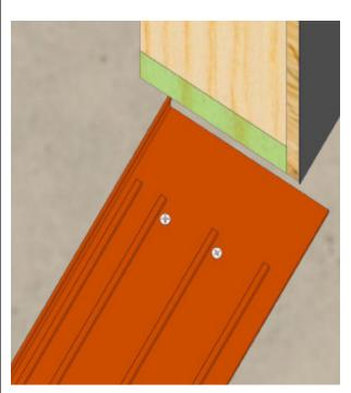
Using a screw with head shorter (less than .150"), screw down the sill pan.
