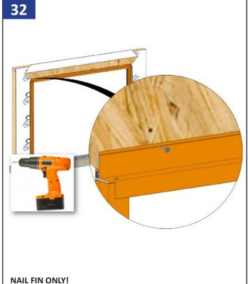
Fully fasten the screws down now to hold the frame in place.
