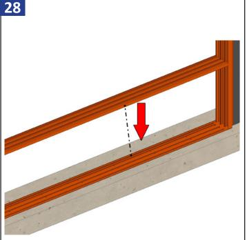
Make sure all foreign material is removed from sill and sill pan(s). Set the sill(s) in place.
