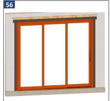
Apply a 3/8" sealant bead to the perimeter edge of door frame before installing the drip cap.
