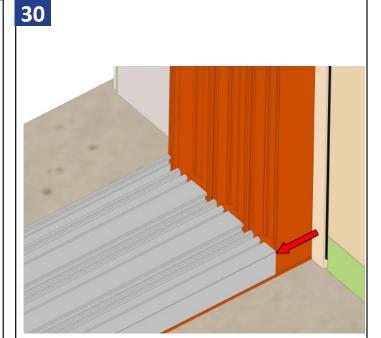
Shim jamb frame to the sill. No more than a 1/16" gap.
