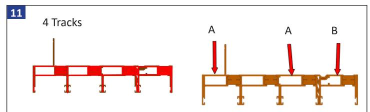
Place a gasket (Part #: QWP-MMSD-V5FG4(B/W)) on each face profile of the frame header. Place 2 of the corner keys (Part #: FE\_25-7x10-35-DT) in both ends of the frame header by arrow (A) and place corner key (Part #: M25762-PCS) by arrow (B). Then join to both frame jambs to head. Trim weather strip flush to both ends.
