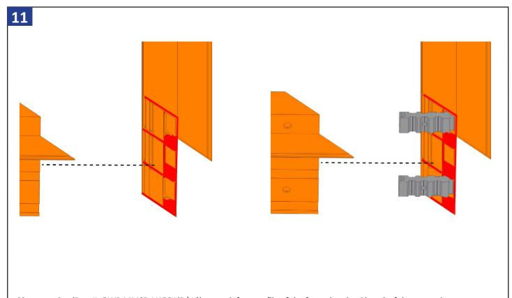
Place a gasket (Part #: QWP-MMSD-V4FG1(B/W)) on each face profile of the frame header. Place 2 of the corner keys (Part #: FE\_25-7x10-35-DT) in both ends of the frame header and join to both frame jambs. Trim weather strip flush to both ends.
