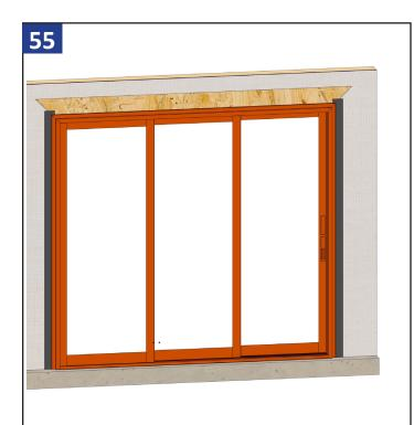
Apply flashing tape at the sides of the door as shown. Smooth using a J-roller. Extend tape a minimum of 2" past door frame, but not more than the thickness of the flashing tape.
