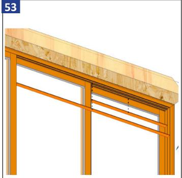
Next install the short and long header covers in the exterior and middle tracks. Trim covers to fit if needed.
