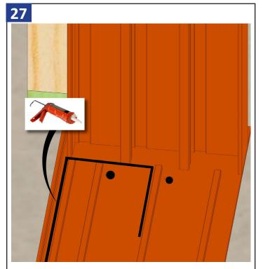
Run a bead of silicone along the wall, up the leg of the sill pan, and along the interior most leg the length of the sill pan.
