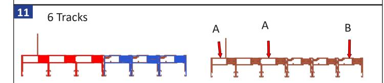
Place gasket (Part #: QWP-MMSD-V4FG1(B/W)) (RED) on the first three tracks, and then place gasket (Part #: QWP-MMSD-V5FG6(B/W)) (BLUE) on the other three tracks. This will go on each face profile of the frame header. Place 2 of the corner keys
