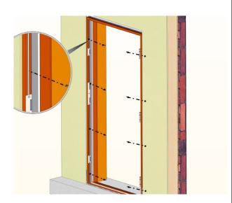
Open the Door and drill a countersink hole through the jambs in the exterior track per anchorage calculations. Quaker Window Products does not supply or claim liability for anchorage/fastener calculations. It is the installer/client's responsibility for structural adequacy of the anchorage and fasteners. Typically, 3" from the corners and 16" on center.
