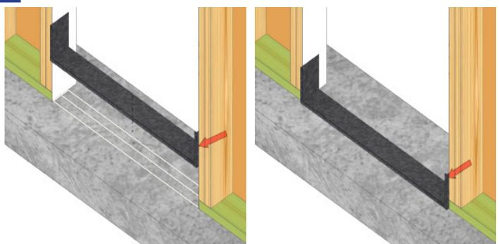
Install a sill pan flashing (by others). If installing the door flush with the interior to allow for a 180 degree door swing make sure to set the sill pan flush with interior wall finish.
