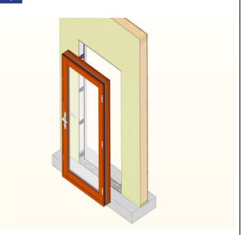
Center and set the door frame into the rough opening. Make sure to keep the door flush with the interior wall finish. Level at the sill and plumb the frame. Shim under the frame to bring to level in necessary.
