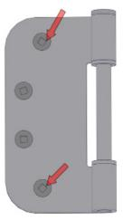
Remove the top and bottom fasteners from the hinge, and drill a clear hole through the frame, to install fasteners into the condition. This needs to be done at every hinge on the door.
