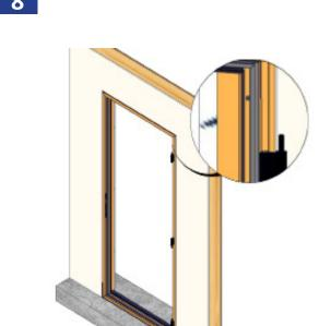
Install and fasten the door unit in place using fasteners by others per anchorage calculations. *Quaker Window Products does not supply or claim liability for anchorage/fastener calculations. It is the installer/client's responsibility for structural adequacy of the anchorage and fasteners.*
