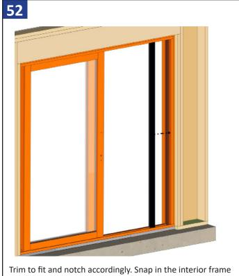
Trim to fit and notch accordingly. Snap in the interior frame jamb filler cover (Part #: BRS-9086) in the inactive frame jamb.
