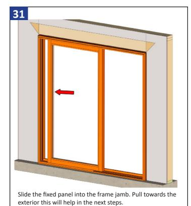
See above diagram. Be sure the fixed panel is seated fully into the frame jamb.
