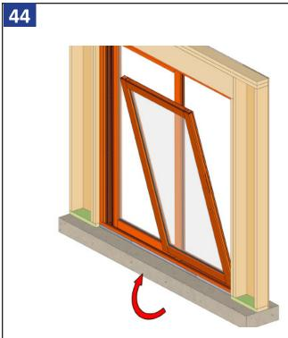
On the interior side set the active panel on the roller track. Make sure the panels are overlapped when installing so the interlocks will engage properly. Slide panel to the fixed jamb. Make sure the closure captures active panel and operates properly.
