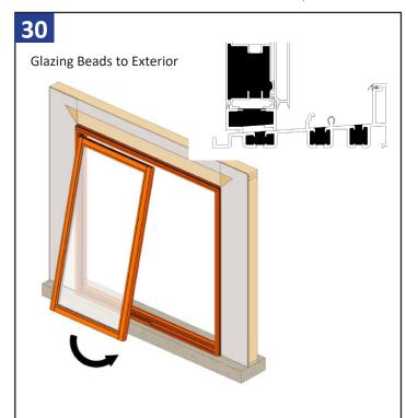
From the exterior, install the fixed panel with the setting chair, by tilting the top into the exterior most head track. Set the bottom of the fixed chair against the lip of the sill.
