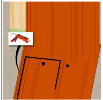
Run a bead of silicone along the wall, up the leg of the sill pan, and along the interior most leg the length of the sill pan.
