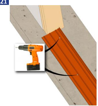
Locate second and third leg and drill holes directly behind them. Drill holes through the sill pan, 3" from each end and then 14" on center for the length of the pan, alternating between the 2 tracks.
