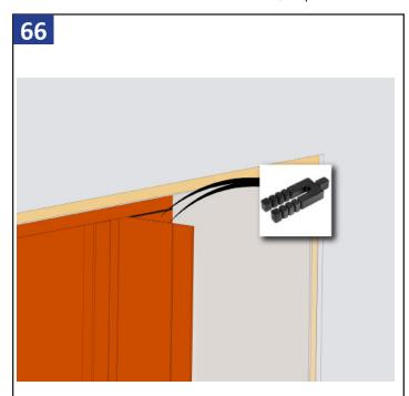
Shim the interior closure out so that the panel and closure seals.
