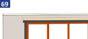
Apply a 3/8" sealant bead to the perimeter edge of door frame before installing the drip cap.
