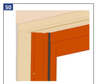
Take the exterior closure interlock (Part #: M25389) and cut it to length. Lock the door system. Rough fit it in the opening, and shim if necessary. If unable to lock, the closure needs to be shimmed out toward the lock.
