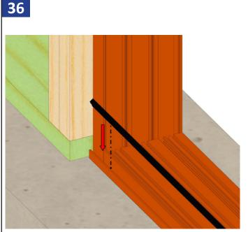
Locate the interior side of the sill. Push the sill down and towards the exterior to lock in place. Take the wedge gasket (Part #: 4874-02-00) and press in place.
