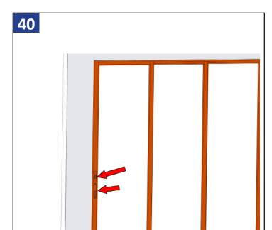
Adjust active panel level, get to lock and then adjust other panels. (The active panel is the panel with the handle set, and the interior most panel.)
