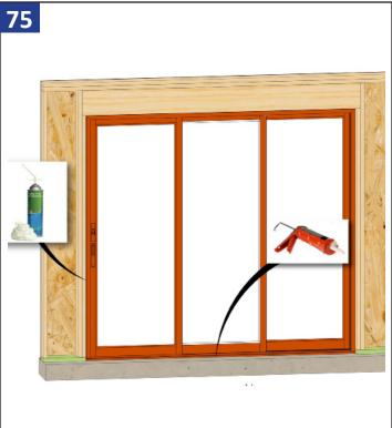
Insulate the gap between the door and framing with minimally expanding spray foam, and seal the entire interior perimeter with sealant.
