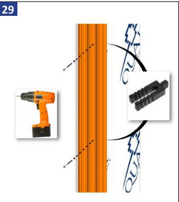
Temporarily set screw just deep enough to hold the frame in place. The screws through the center track of the header & jambs, typically 6" from ends and 24" on center for fasteners.
