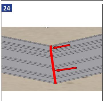
Apply silicone where the 2 sill pans meet, up the interior most leg, and makes a 90 degree corner. Make sure this joint is tight.
