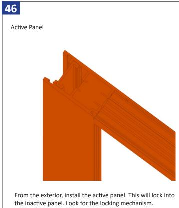
\*Note orientation of interlock rails when choosing panels. \*Note glazing beads are to the interior side.
