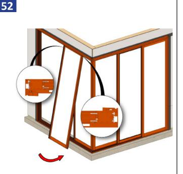
On the exterior side repeat for the middle panel, setting it into the middle tracks in the head and sill. Make sure the panels are overlapped when installing so the interlocks will engage properly.
