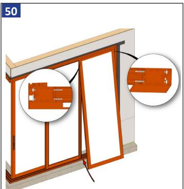
Repeat for exterior panel, setting it into the exterior tracks in the head and sill. Make sure the panels are overlapped when installing so the interlocks will engage properly.
