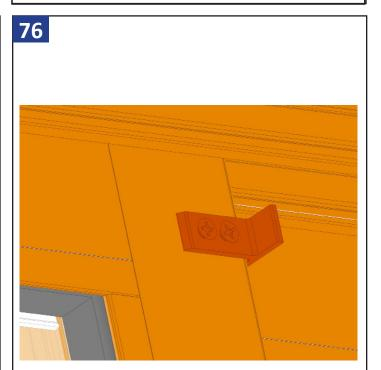
On the interior side of the middle panels, take the panel pickups (Part #: M25296-PCS) and #10 screw (Part #:MF10AX1)that is provided. Take screws and attach the pickups. Install the panel pickup where the holes are already fabricated on the interior side of the door. wd
