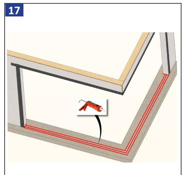
Apply three 3/8" continuous beads of sealant across the entire width of the rough opening sill where the sill pan will sit. Be sure to make a continuos path around the corner as shown above. Apply two 3/8" continuous beads of sealant the width of the pan, 1/2" from each side of opening as shown above.
