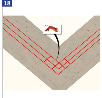
On each side of the 90 degree corner apply 2, 3/8" beads of silicone across the 3 beads of silicone as shown above.
