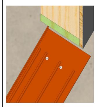
Using a screw with head shorter (less than .150"), screw down the sill pan. Check to make sure sill pan is still level. Shim accordingly.
