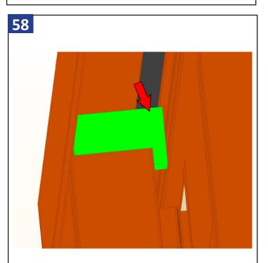
Slide the fix panel fully into the frame jamb, then take the frame head dust plug and remove backing. Slide the dust plug in between the head and the top of the fixed panel. The edge of the panel and the face of the dust plug should be flush.
