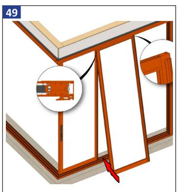
On the exterior side repeat for the middle panel, setting it into the middle tracks in the head and sill. Make sure the panels are overlapped when installing so the interlocks will engage properly.
