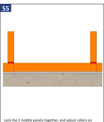
Lock the 2 middle panels together, and adjust rollers on all panels so they roll smoothly. Start with the 2 hardware panels and work your way towards the fixed panels. Check the reveal of the glass at the bottom of panels and adjust as needed to line up all panels.
