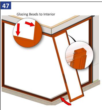
From the exterior, install the locking panel with the handle, by tilting the top into the inner most head track and setting the bottom of the panel in the inner most groove in the sill track.
