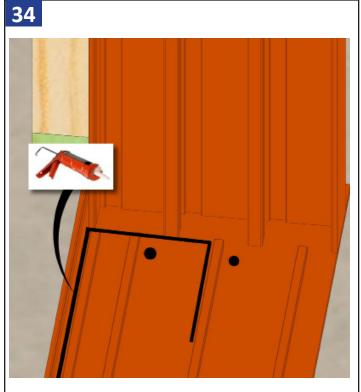
Run a bead of silicone along the wall, up the leg of the flashing pan, and along the interior most lip. Note: This will be the space between the lip of the flashing pan and the first leg, as shown above.
