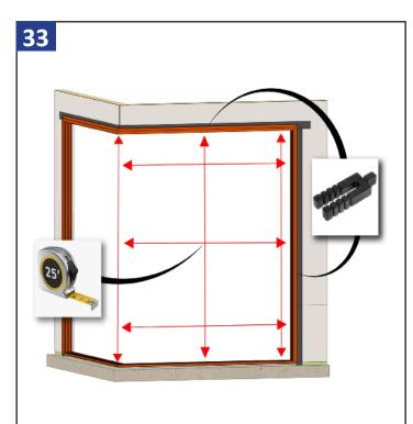
Take other side of the frame and slide it onto the 90 degree keys in the head.
