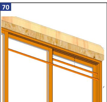
Next install the short and long header covers in the exterior and middle tracks. Trim covers to fit if needed. DO NOT HIT THE HEADER COVERS DIRECTLY DURING INSTALL! NOTE: ON ACTIVE PANEL MEASURE FROM PANEL TO FRAME AND SUBTRACT 1/16", CUT, THEN PLACE AGAINST FRAME.
