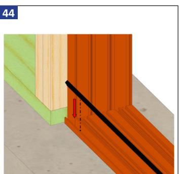
Locate the interior side of the sill. Push the sill down and towards the exterior to lock in place. Take the wedge gasket (Part #: 4874-02-00) and press in place. Note: This will run the whole length of the sill pan.
