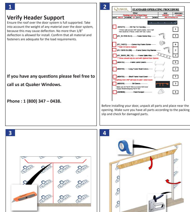
Apply the house wrap according to the manufacturer's instructions and cut T-pattern opening as shown above. Cut top flap angles at 45 degrees and 1" longer than the width of flashing tape being used.
