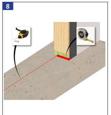
Measure and set a chalk line on the sub floor 4 7/8" in from the exterior wall face. Dry fit the provided sill pan system with the rear upturned leg on this line. **The sill condition must be level.**
