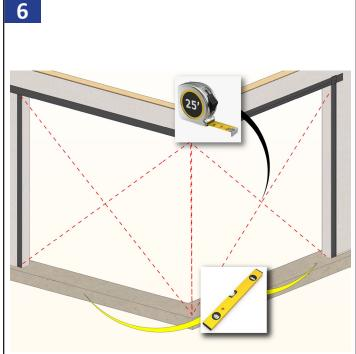
Check that the opening is square. The diagonal measurements need to be within 1/8" of each other. Verify the rough opening is plumb and level.
