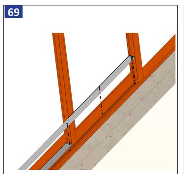
Next install the exterior sill cover. DO NOT HIT THE SILL COVERS DIRECTLY DURING INSTALL! NOTE: ON ACTIVE PANEL MEASURE FROM PANEL TO FRAME AND SUBTRACT 1/16", CUT, THEN PLACE AGAINST FRAME CUT LONG YOU CAN ALWAYS CUT MORE OFF! **REPEAT FOR THE OTHER SIDE.**
