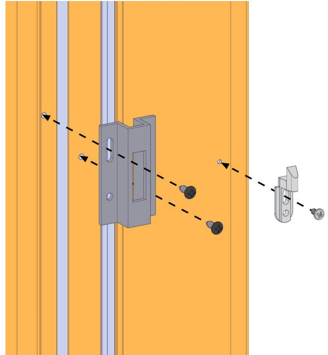
Install meeting rail lock keepers for the active panel and screen door. Use pre-punched holes in the meeting rail to align with the slotted holes in keepers.
