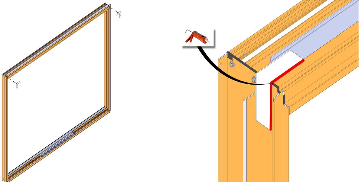
Clean the nail fin corners with 99% isopropyl alcohol prior to installing the corner gaskets to the exterior side of nail fin corner gaps. Apply sealant along the edge where the gasket meets the door frame as shown.
