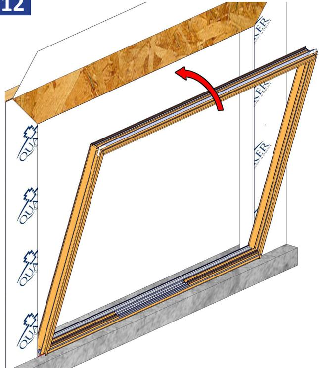
Center and set the door frame into the rough opening, making sure there are equal gaps on both sides of the door.
