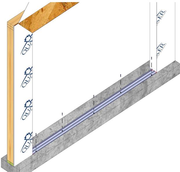
Fasten sub-sill anchor plate as shown above.
