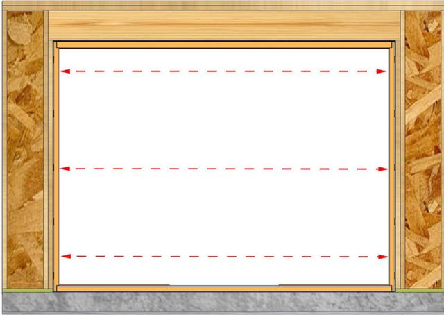
Check that the door frame is not bowed. Adjust shims as needed until measurements are within 1/8".
