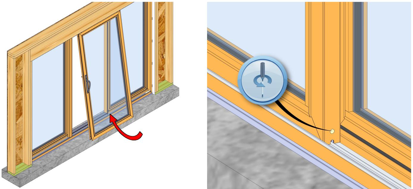
Angle the active panel with the top inserted into the head track, and then lift and set the bottom rollers on the roller track. Use a Phillips #3 screwdriver to adjust the rollers as needed to ensure the panel is level, square, and slides smoothly. Lift on the panel while adjusting, do not use a drill to adjust.
