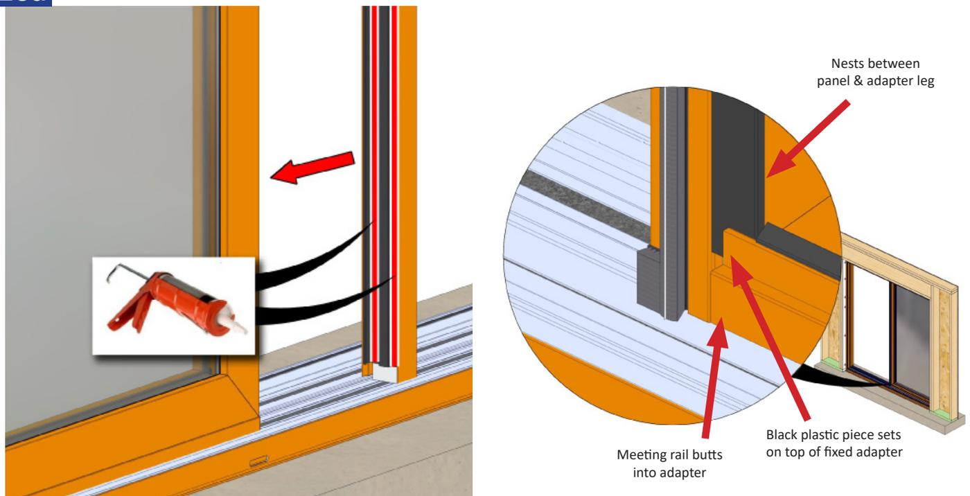
Apply a bead of sealant to inside edges of meeting rail before sliding the pre-assembled meeting rail against the fixed panel. Please see steps 26b and 26c for series specific guidelines.
