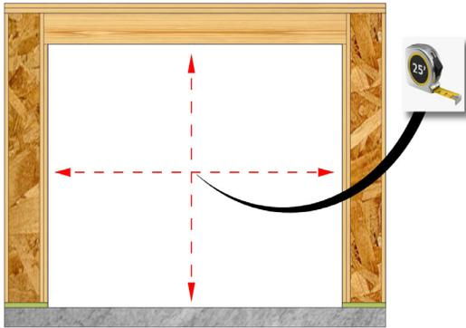
Measure and verify the rough opening is sized correctly. The rough opening should be  $3/4$ " wider and  $1/2$ " taller than the unit. Allow additional space for flashing thickness, installation clips, joining components, and their fasteners.
