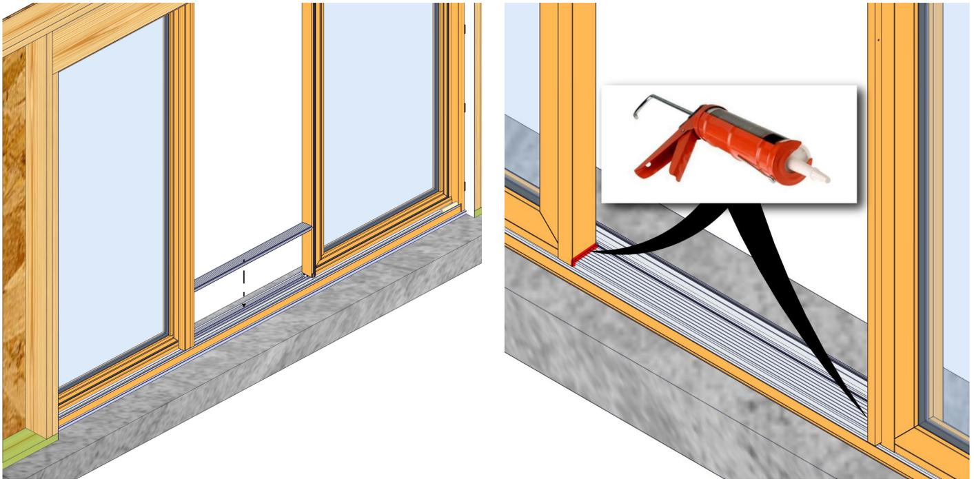
Install threshold on the exterior side of frame covering the bottom angle brackets. Seal around the two ends of the threshold against the frame.
