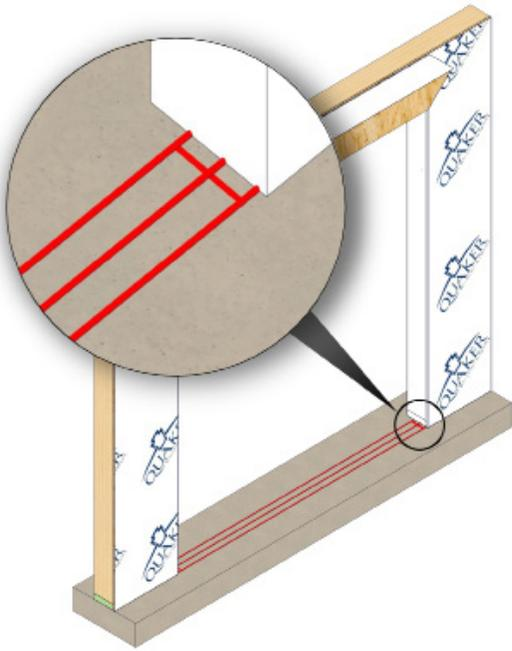
The sub-sill anchor plate will set  $4 \frac{1}{16}$ " in from the exterior face of wall framing. Apply three  $\frac{3}{8}$ " continuous beads of sealant across the entire width of the rough opening sill where the sub-sill anchor plate will set. Apply two  $\frac{3}{8}$ " continuous beads of sealant the depth of the anchor plate,  $\frac{1}{2}$ " from each side of opening as shown above.
