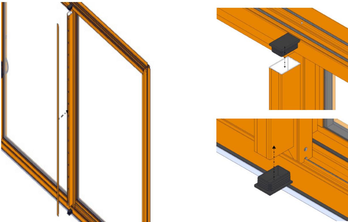
Install reinforcing cover and end caps to reinforcing tube.
