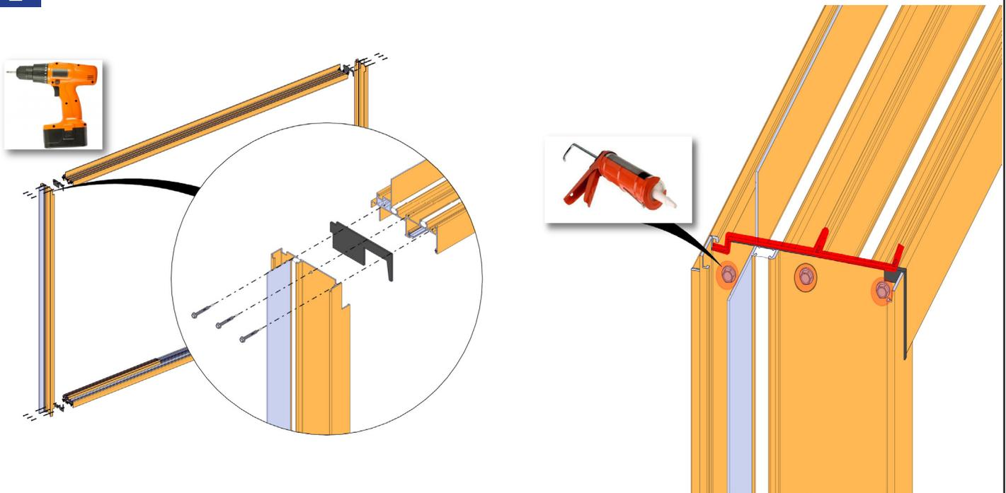
Apply the head and sill gaskets to each end of the head and sill. Assemble jambs to head and sill assembly with the 12 fasteners provided (MH8-18X11/2 LP) and seal around all screw heads, exposed screw threads, and outside corners.
