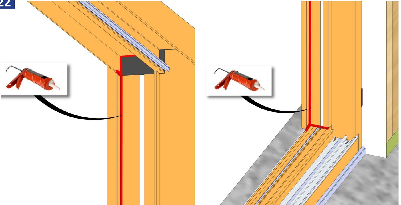
Seal the inside edge corners at the head, sill, and jamb where the fixed panel will set in the frame, as shown above.
