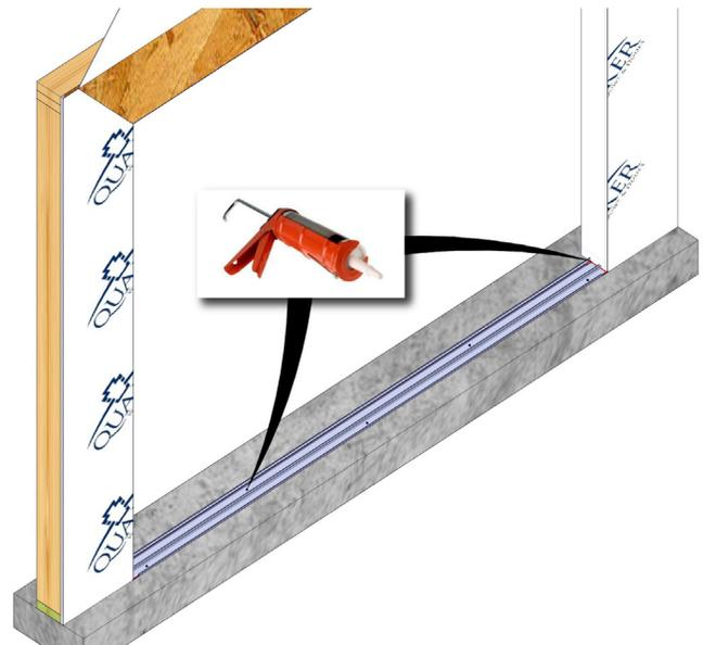
Apply sealant over fastener heads and at the ends of the sub-sill anchor plate where the plate meets the wall framing.
