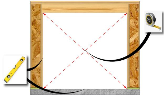
Check that the opening is square. The diagonal measurements need to be within  $1/8$ " of each other. Verify the rough opening is plumb and level. **The sill plate beneath the unit must be level for proper unit operation.**
