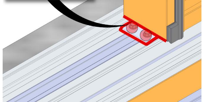
For all other M-Series units, install the pre-assembled meeting rail against the fixed panel and install using supplied (MH8-18X1/2 TK2) screws in the head and sill angle brackets. Apply sealant over the screw heads in the sill and along the perimeter of the angle bracket. Repeat step for the other meeting rail.
