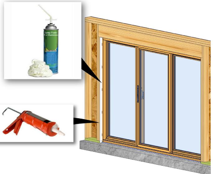
Fill interior 1/3 of cavity using low expanding foam or backer rod and apply sealant continuously around entire perimeter of opening.
