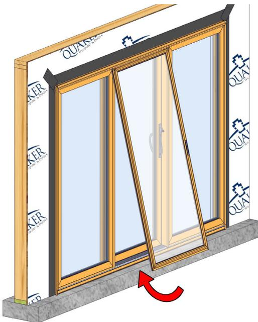
Angle the screen panel with the top inserted into the head track, and then lift and set the bottom rollers on the roller track. Adjust rollers as needed to insure the panel is level, square, and slides smoothly.
