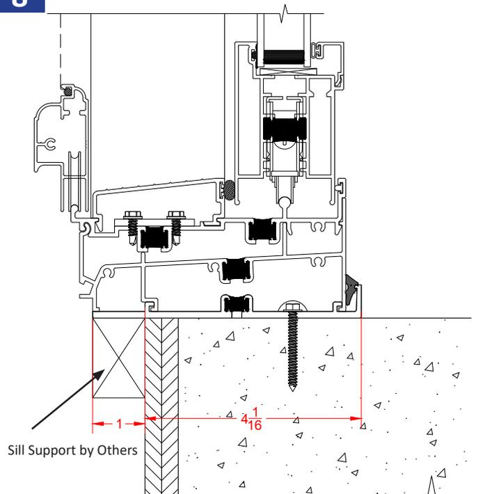
Install the sub-sill anchor plate  $4 \frac{1}{16}$ " in from the exterior face of wall framing.
