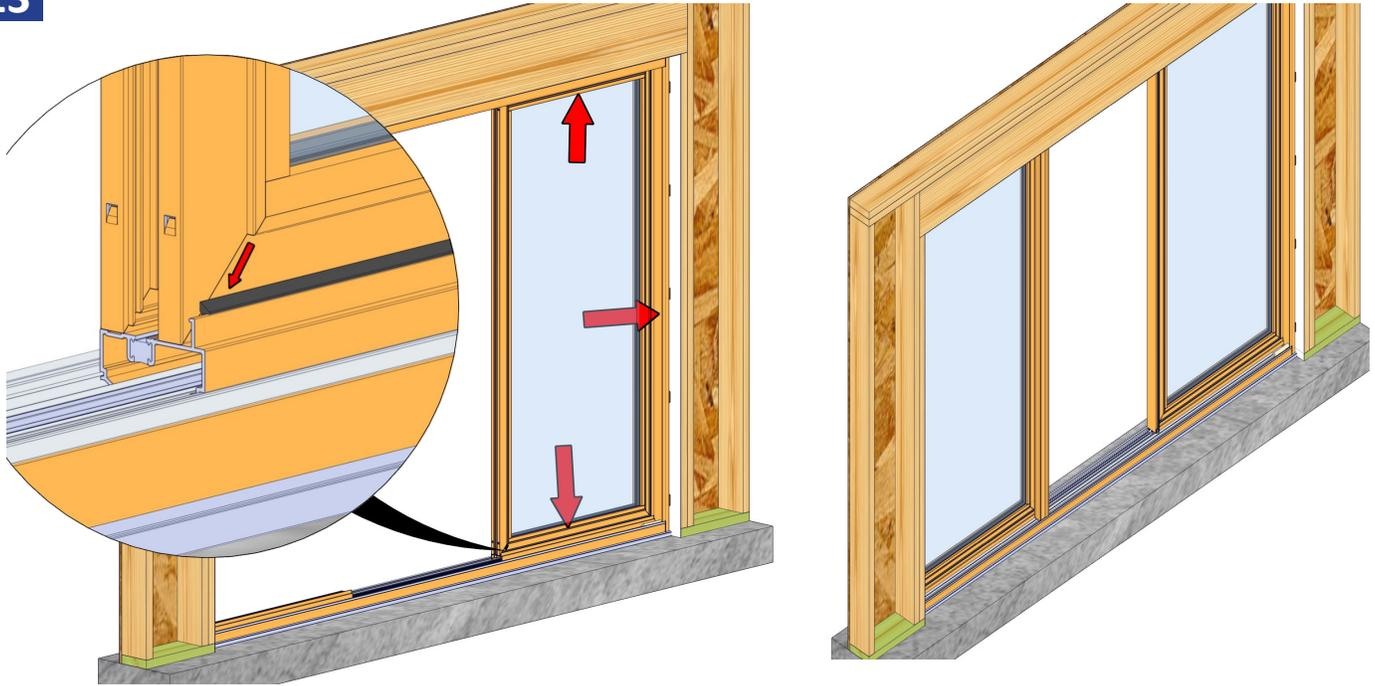
Install wedge gasket in the sill, head, and jamb around the interior of the frame and panel to secure the panel in place. Repeat steps 20, 21, 22, and the first step of 23 for the other stationary panel.
