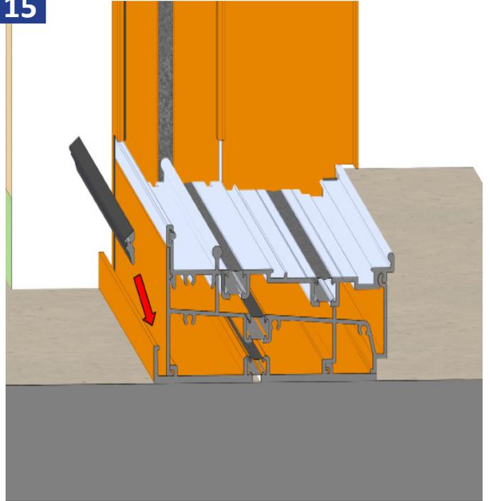
Install the wedge gasket in the sub-sill anchor plate against the interior leg of the door as shown above.
