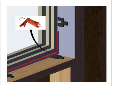
Apply a bead of sealant to fill the gap between the sill pan flashing system and the window unit.
