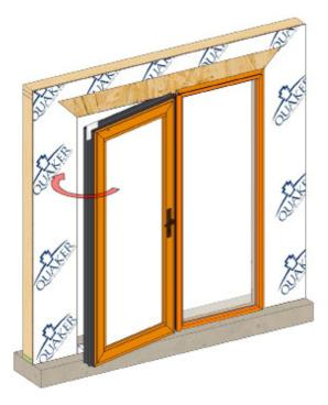
Install door in rough opening, setting in the bottom of the door first, working in to place behind the mull. Verify squeeze out of sealant along positioning fin. Refer to the appropriate door install guide for anchoring door (IG-070 No positioning fin or IG-071 With Positioning Fin) but do not install the door jamb cover on the mull side yet, or the head cover and sill threshold.
