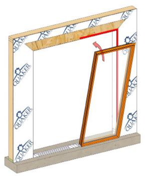
Apply a continuous 3/8" sealant bead at the side and the top of the opening where the window/sidelite will go, no more than 1/2" from the edge of the opening. Install window/sidelite in rough opening, lifting and setting the bottom of the unit in first, then tilting into place. Verify for squeeze out of sealant along nailing fin.
