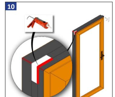
Install the top foam corner key gasket over the exterior side of the positioning fin corner gap on the door. Seal the exterior corner where the gasket meets the position fin as shown above.
