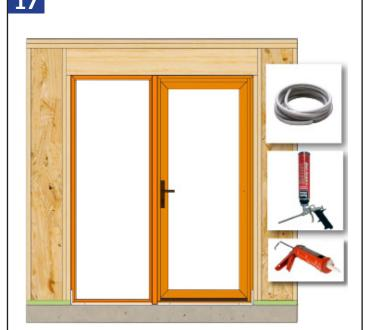
Insulate and seal around the entire perimeter of the window units.
