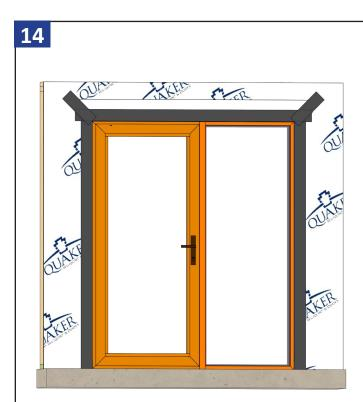
Finish flashing the exterior of the window per Quaker standard nail fin installation guidelines.
