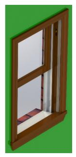
Cut the balance cords on the bottom sash and remove the sash and dispose of it properly. Allow weights to fall to the bottom of the weight pockets.
