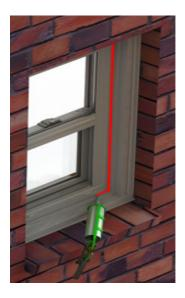
If total frame replacement in brick or siding was preformed maintain a minimum of ¼" between the window frame, trim, siding, or masonry. Apply backer rod (if needed) and a continuous bead of sealant between the window frame and exterior finish material on all four sides of unit. Make sure to clean all surfaces before applying sealant (some surfaces may need to be primed so check with sealant supplier).
