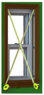
Check for plumb, level, square and window operation. Make any necessary adjustments to shims and finish installing frame screws. Raise bottom sash to install bottom screws, and tilt bottom sash in to install center screws.
