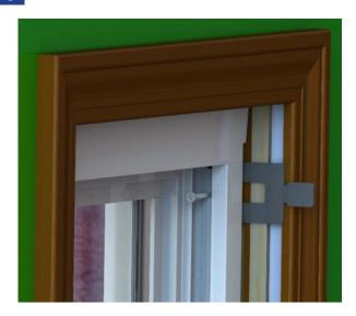
Place a shim at each of the pilot hole locations, and insert a screw into one top corner to hold window in place. Remove sash stop at head of window and replace when screws are tightened. Note: When installing all installation screws make sure to tighten screw so the screw head is flush or slightly dimpled in so screw doesn't interfere with balance shoe.
