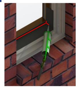
Place a bead of sealant where the existing stool meets the existing window sill. Insert window into the opening. Set the bottom of the window in first and tilt top into place. Make sure the window is centered in opening and press firmly against sealant on blind stops.
