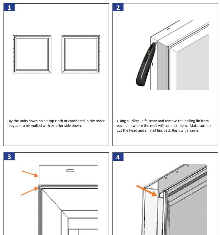
Install the j-channel filler into j-channel slot on the side to be mulled of the exterior of each window. Cut the filler short of head and sill j-channel slot so as not to obstructed the channel.
