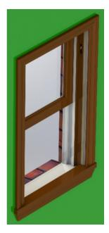
Cut the balance cords on the bottom sash and remove the sash and dispose of it properly. Allow weights to fall to the bottom of the weight pockets.
