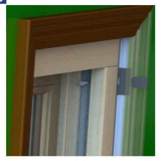
Place a shim at each of the pilot hole locations, and insert a screw into one top corner to hold window in place. Remove sash stop at head of window and replace when screws are tightened. Note: When installing all installation screws make sure to tighten screw so the screw head is flush or slightly dimpled in so screw doesn't interfere with balance shoe.
