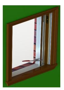
Remove the jamb and head parting stops (if applicable) by pulling or prying them out of the frame.
