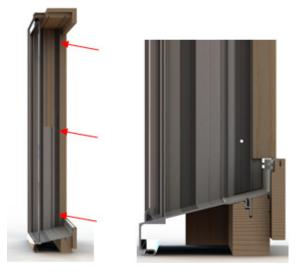
Drill pilot holes (if necessary) in the new window frame. Plan ahead for all holes especially the top of jamb. Make sure top pilot hole will not be in the same locations as the weight pulleys. Use a 1/8" drill, and minimum of 3 holes per jamb. Place holes in center of inside balancer track minimum of 3" from corners, and one in center of the check rail. Tilt the bottom sash in or remove it to place the center pilot hole.
