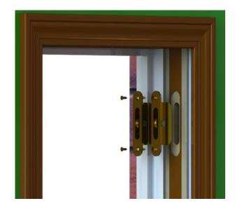
Lower the top sash and cut the balance cords. Remove the top sash and dispose of it properly. Remove the balance chord pulleys. Remove any remaining jamb liner material (if applicable). Insulate the weight pockets and any openings or voids.
