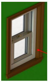
Insulate between the window frame and the rough opening using minimally expanding window and door spray foam or fiberglass insulation. Operate window unit to ensure proper operation. Sash will not operate correctly if window is out of square, over-shimmed or over-insulated. Allow foam to fully cure before installing interior trim. Install interior stops that were remove earlier or cut new stops.
