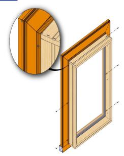
Install self tapping screws around the perimeter of BMC attaching it to the window frame as shown above.
