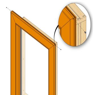
Apply a screw in each of the top corners of the BMC to hold the mitered corners together.
