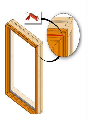
Apply a small amount of sealant inside the mull kerf at the head and down both side jambs.
