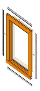
If using the nail fin snap it into the kerf on the BMC and sill nose.
