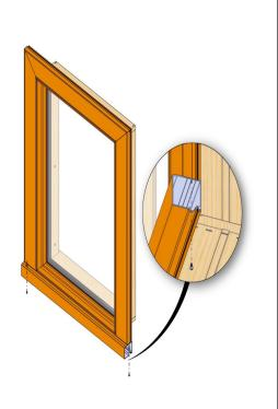
Install two screws through the sill nose into the BMC screw boss as shown above.
