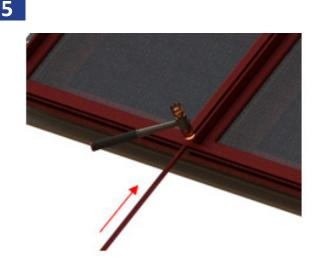
Cut the C-mull keys to the length of the unit (width or height) to be mulled.
